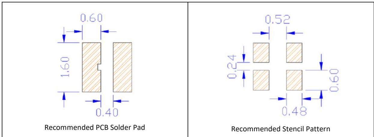
1. Dimensions are in millimetre (mm).
