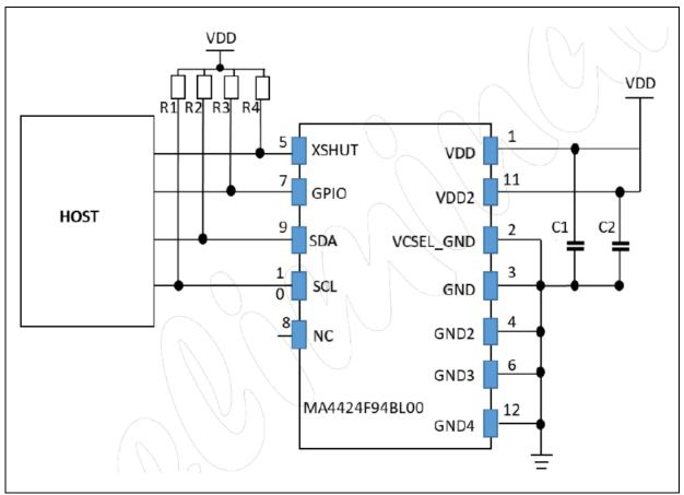
Figure 9. Application Schematic
