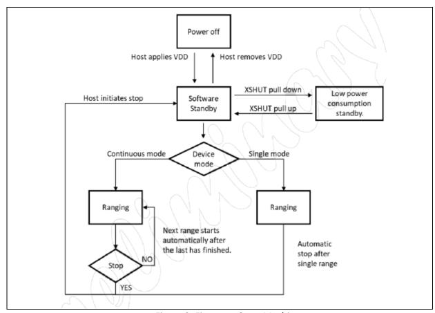
Figure 2. Firmware State Machine
