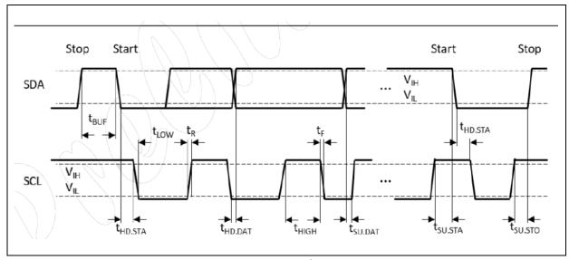
Figure 8. I2C Timing Characteristics
