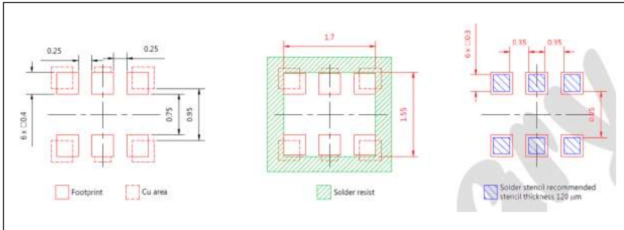
1. Dimensions are in millimetre (mm).
