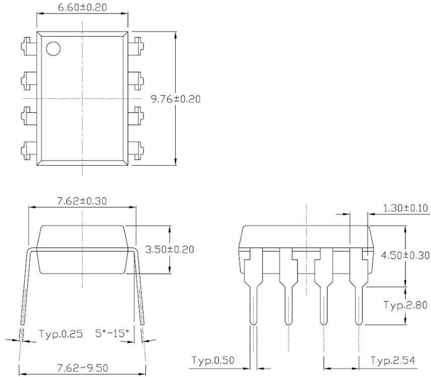
**Gullwing (400mil) Lead Forming – Through Hole (M Type)**
