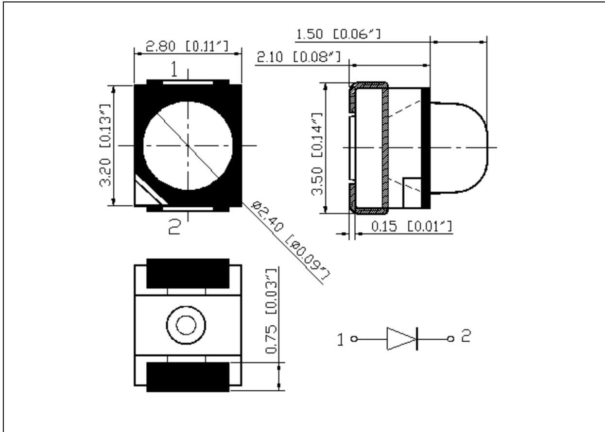
1. All dimensions are in millimetre (mm).
