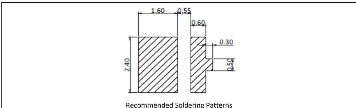
1. Dimensions are in millimetre (mm).
