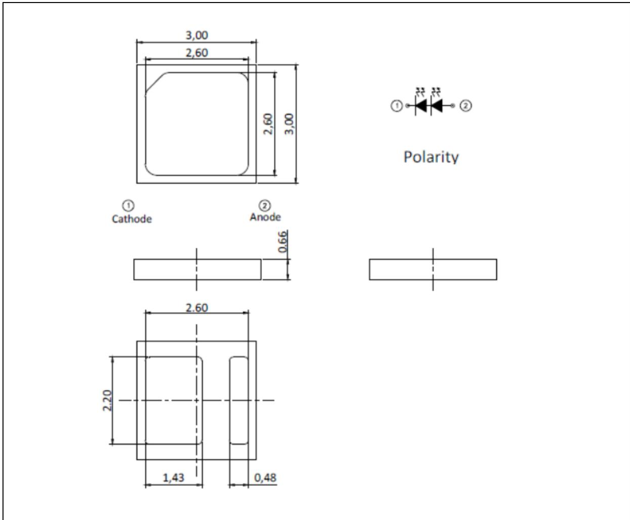
1. All dimensions are in millimetre (mm).
