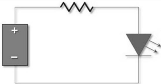
Must apply resistor(s) for protection (over current proof).
