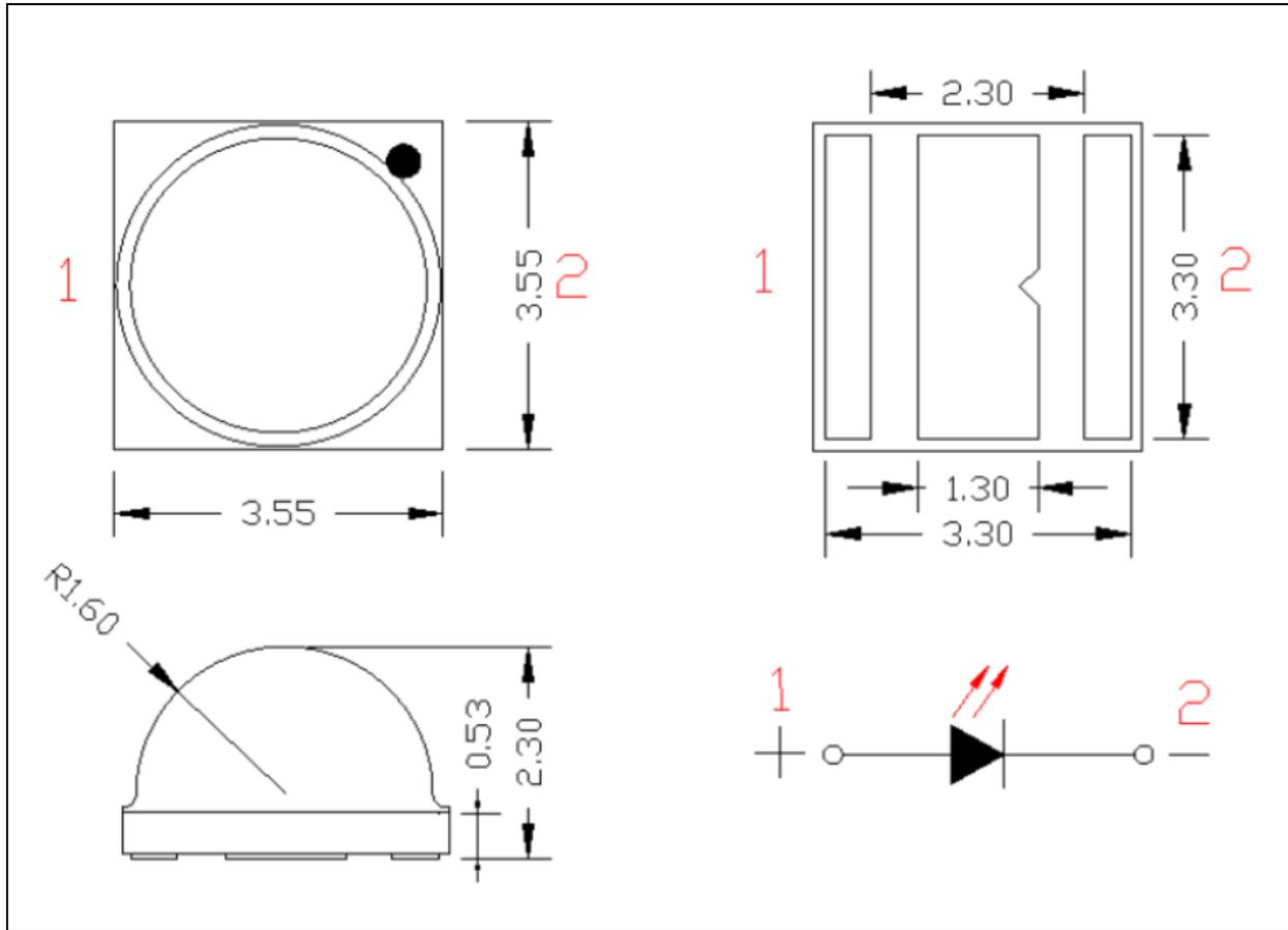
1. All dimensions are in millimetre (mm).
