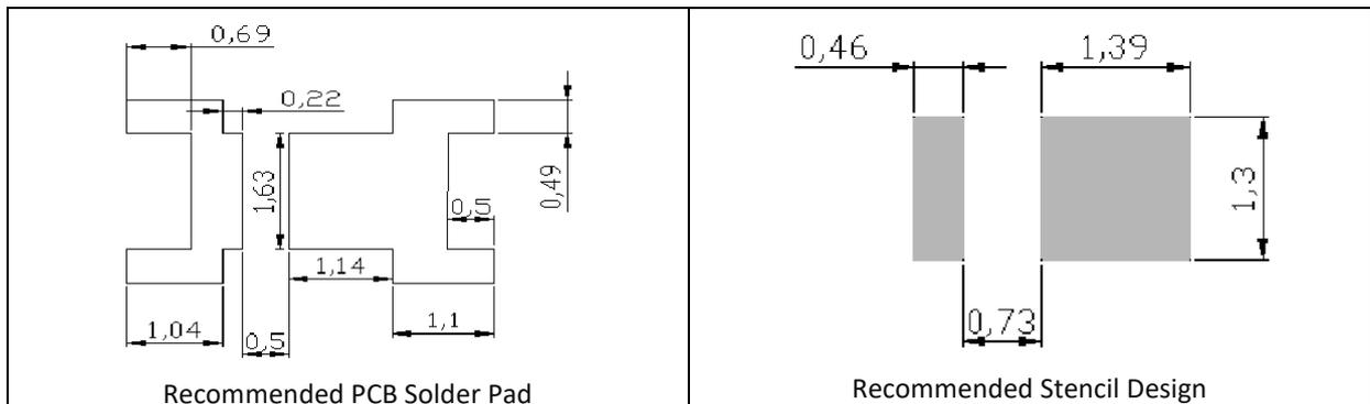
1. Dimensions are in millimetre (mm).
