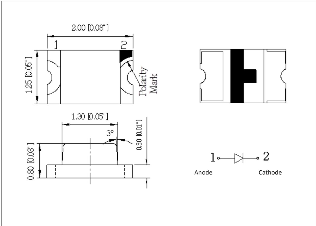
1. All dimensions are in millimetre (mm).
