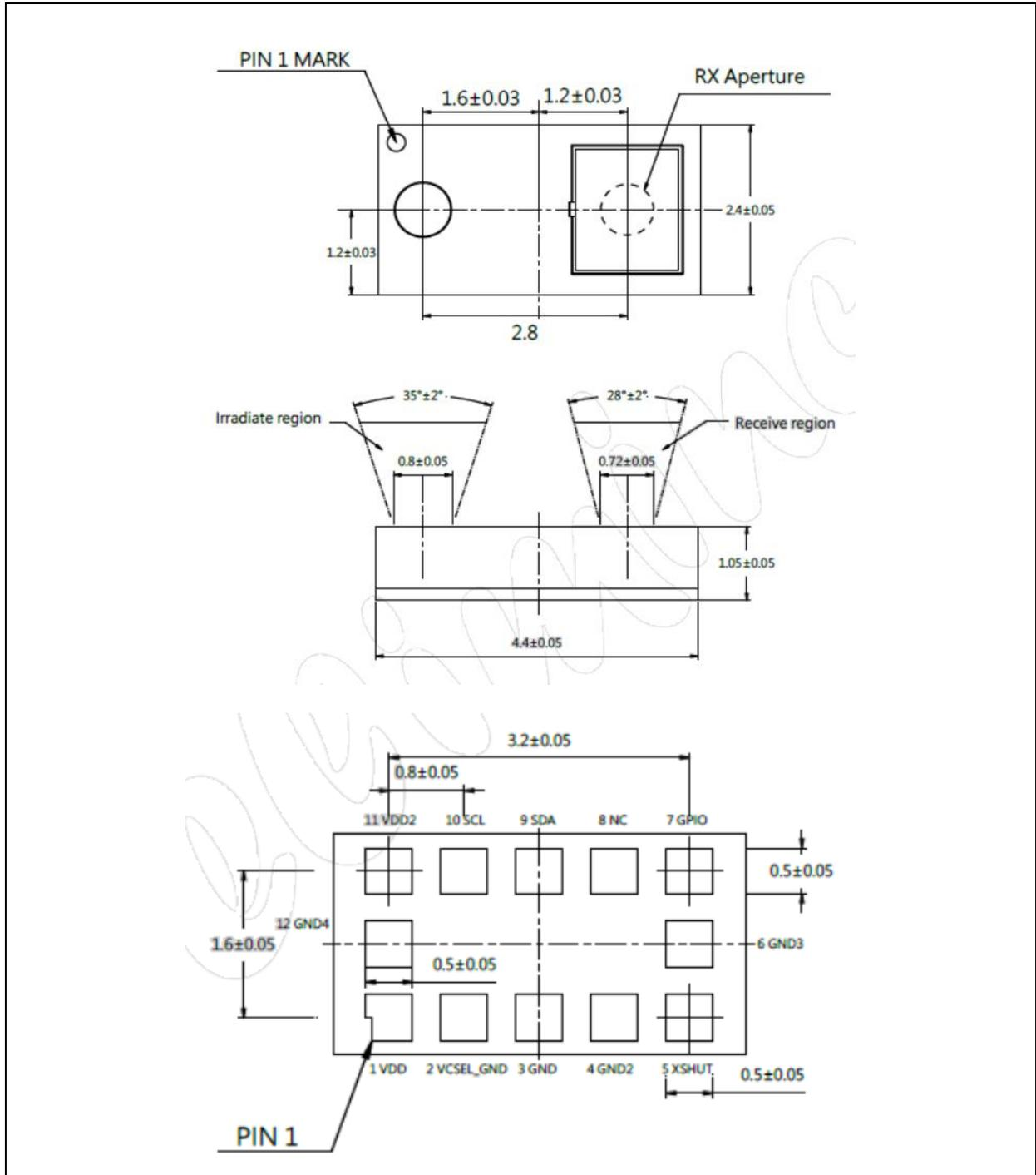
1. All dimensions are in millimetre (mm).
