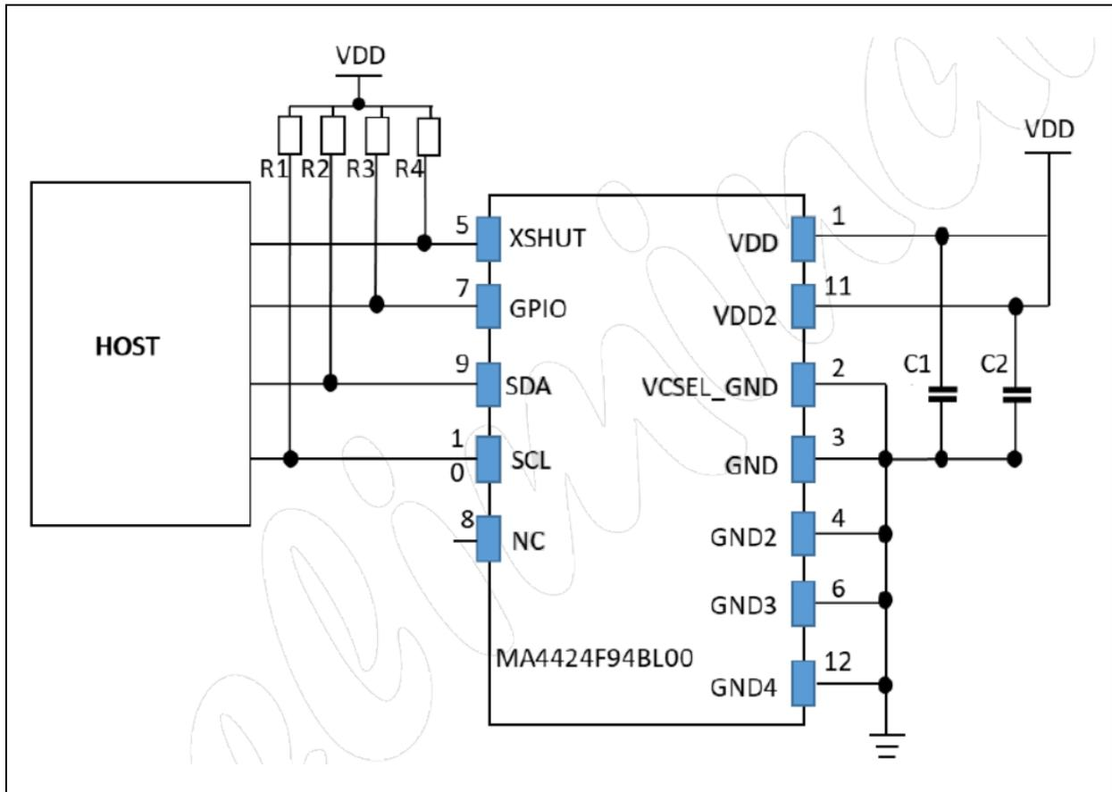
Figure 9. Application Schematic
