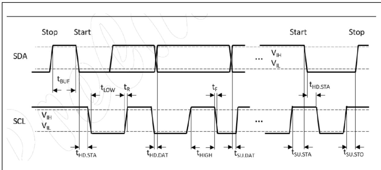
Figure 8. I2C Timing Characteristics
