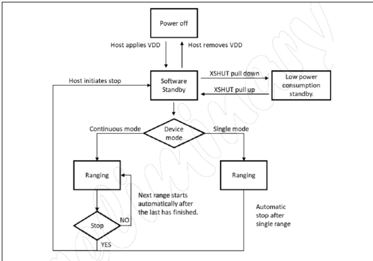
Figure 2. Firmware State Machine
