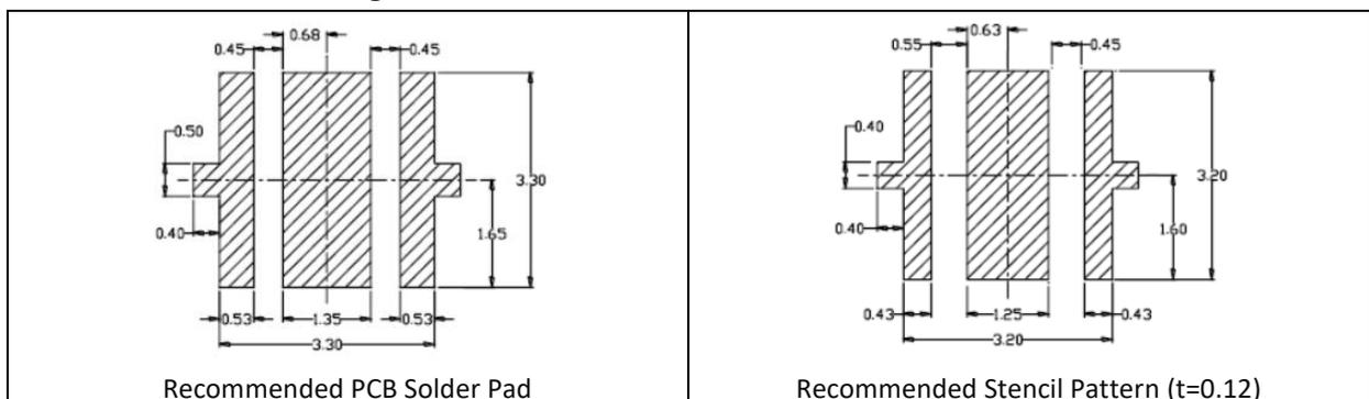
1. Dimensions are in millimetre (mm).
