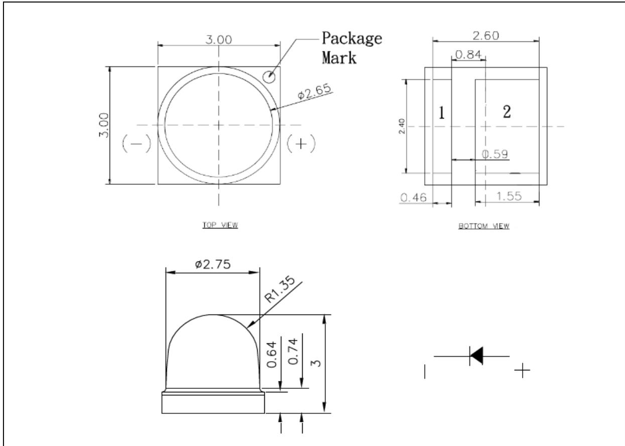
1. All dimensions are in millimetre (mm).
