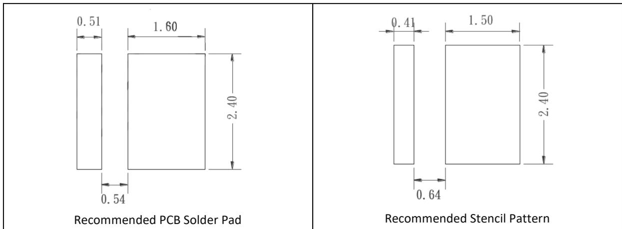
1. Dimensions are in millimetre (mm).
