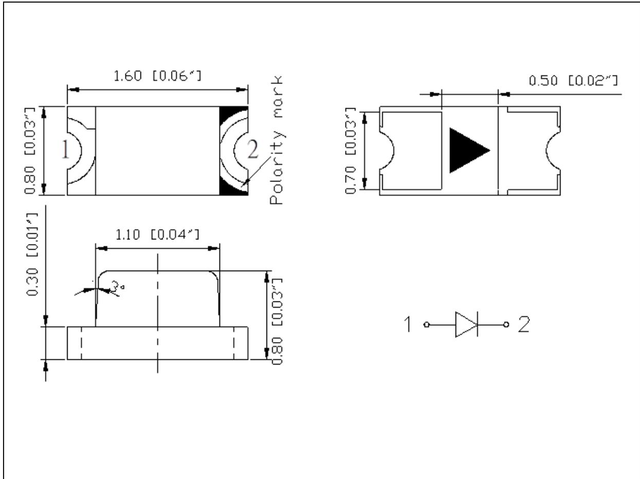
1. All dimensions are in millimetre (mm).
