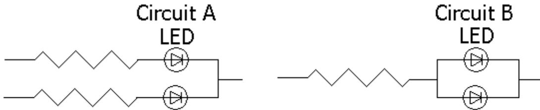
(a) Circuit A it is recommended circuit.
