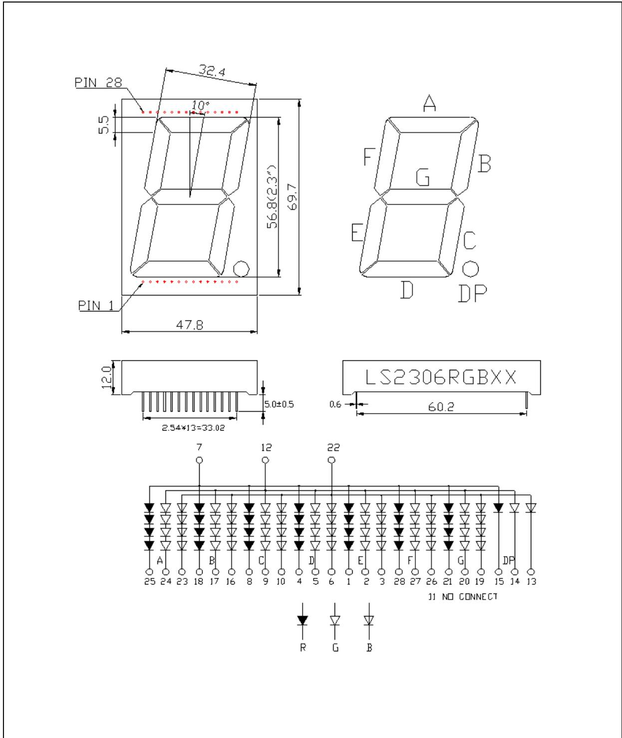
1. All dimensions are in millimetre (mm).
