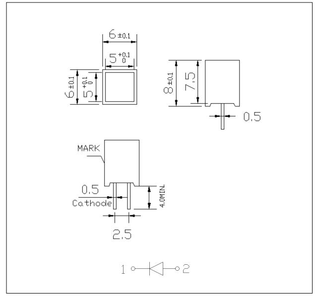
1. All dimensions are in millimetre (mm).
