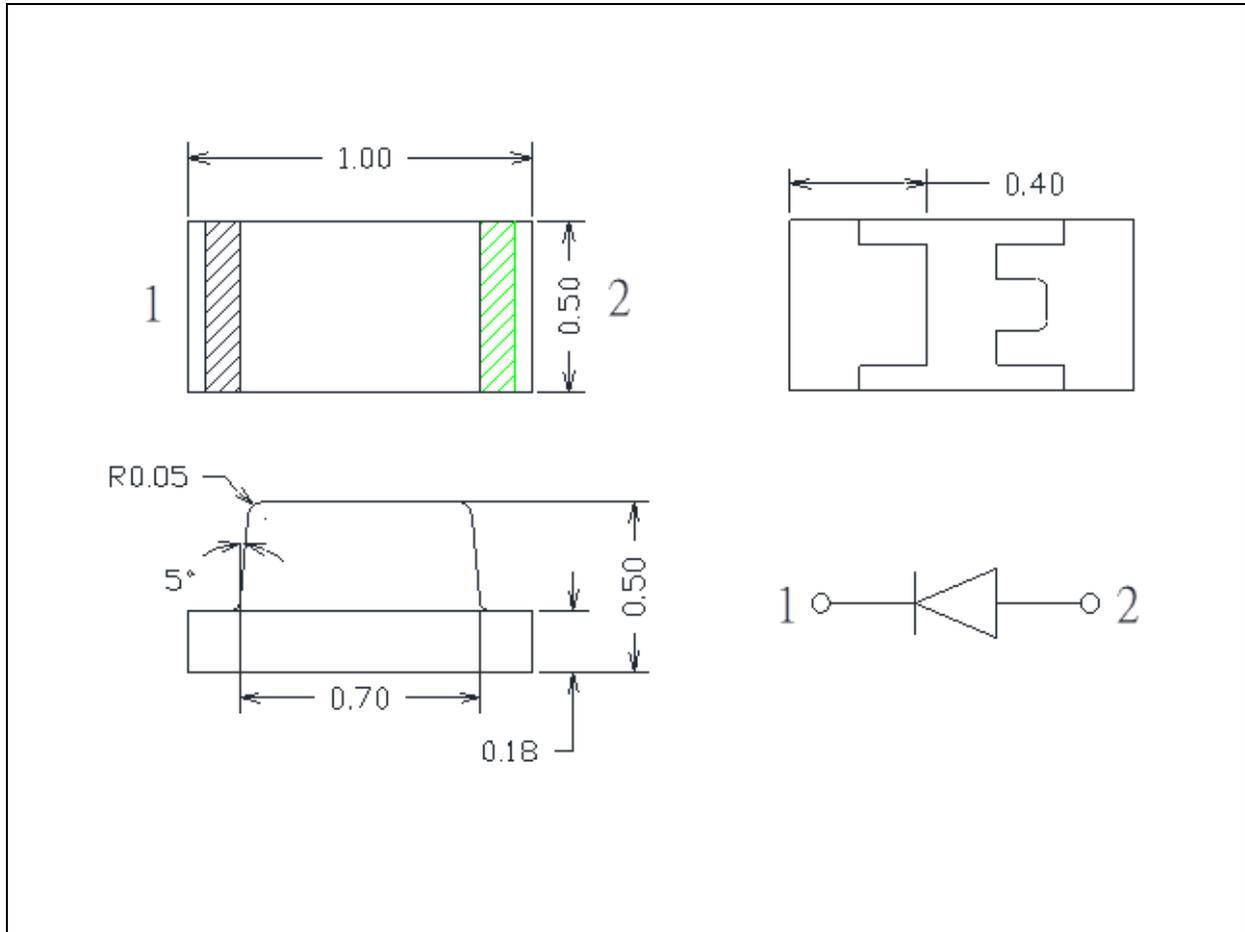
1. All dimensions are in millimetre (mm).
