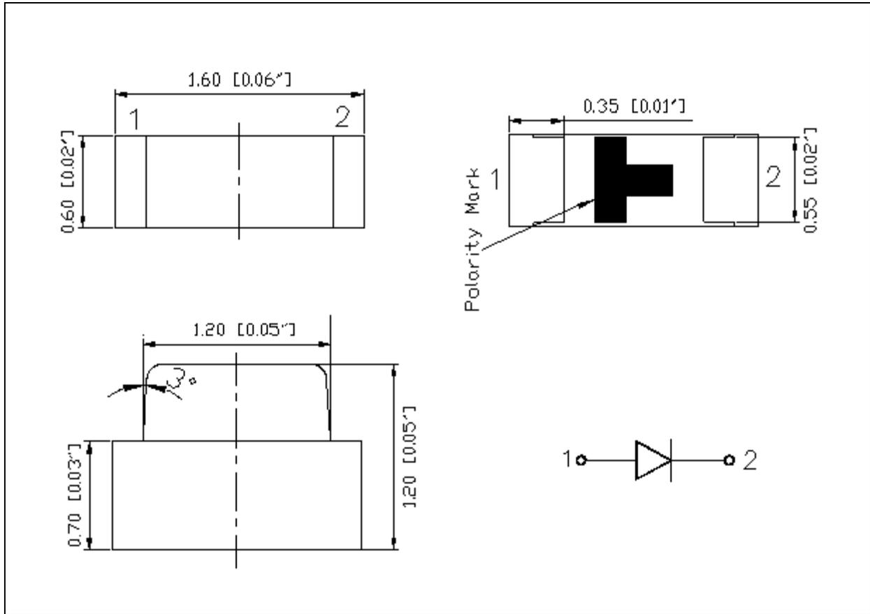
1. All dimensions are in millimetre (mm).
