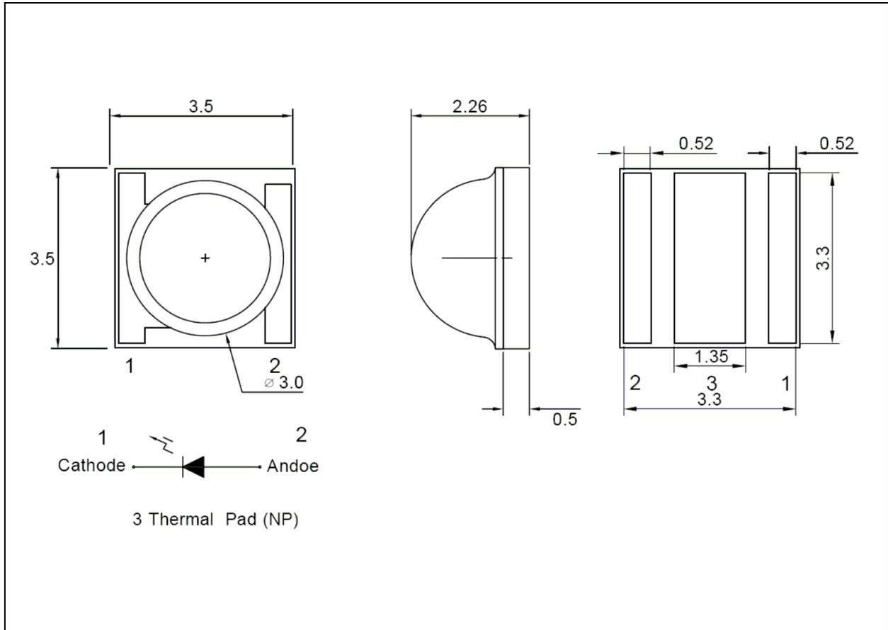
1. All dimensions are in millimetre (mm).
