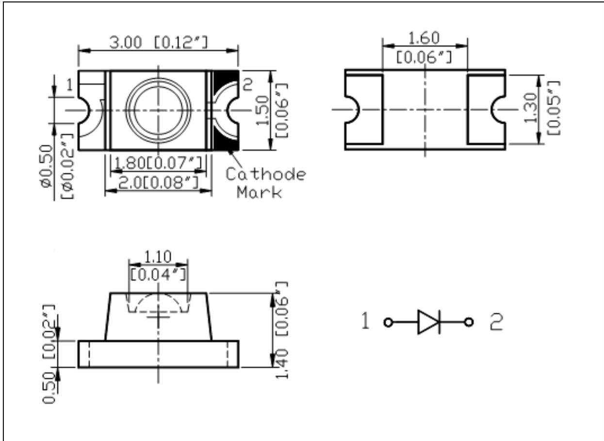
1. All dimensions are in millimetre (mm).
