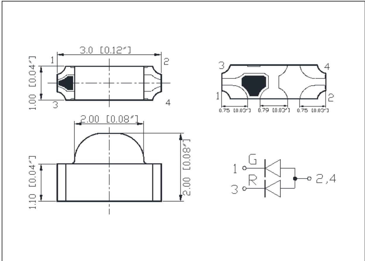
1. All dimensions are in millimetre (mm).
