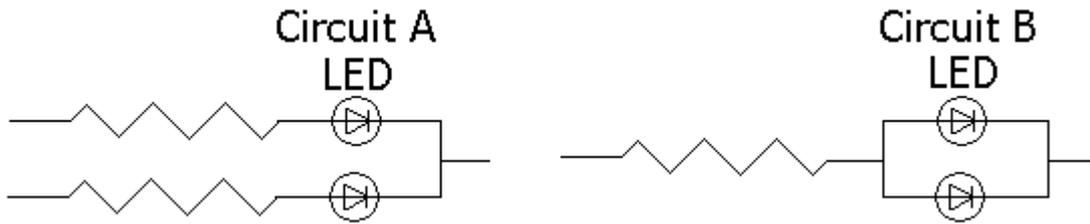
(a) Circuit A it is recommended circuit.
