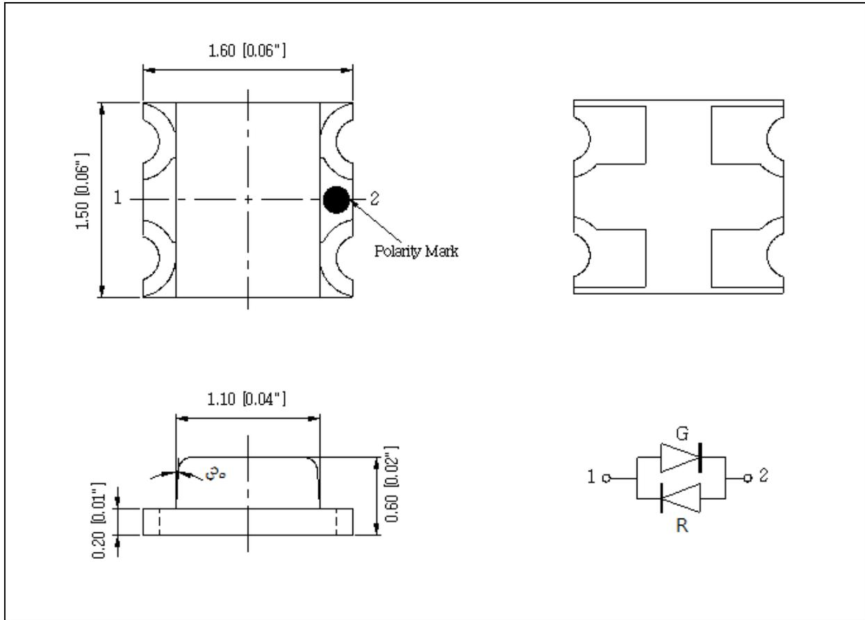
1. All dimensions are in millimetre (mm).
