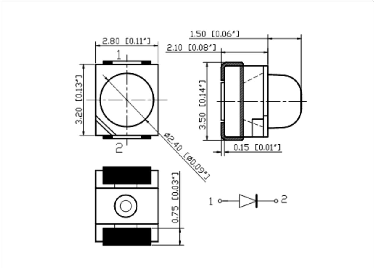
1. All dimensions are in millimetre (mm).
