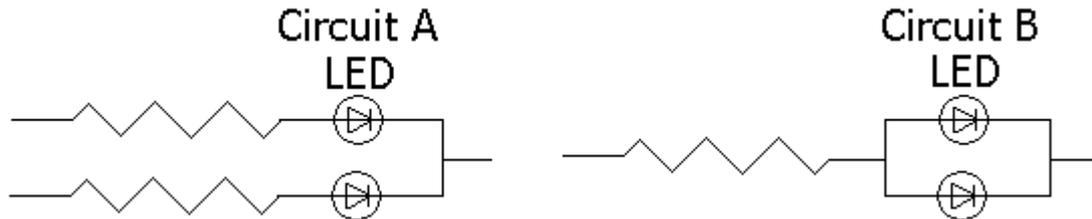
(a) Circuit A it is recommended circuit.
