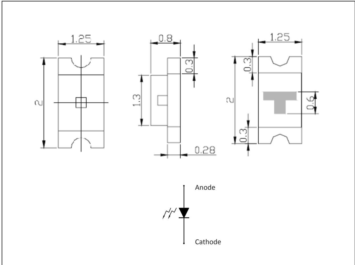
1. All dimensions are in millimetre (mm).
