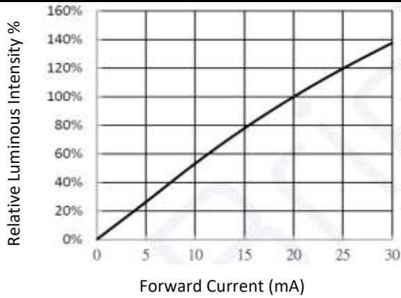
Relative Luminous Intensity v.s. Forward Current
