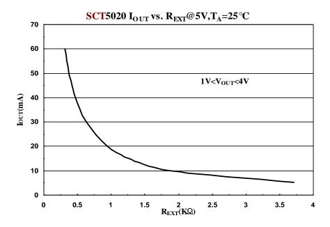
According to I-V curve of the output of SCT5020, the output voltage should be larger than 1V to get 45 mA constant current. By applying proper output voltage, the output current set by an external resistor is approximate to:  $I_{OUT} = 30(615 / REXT)$  (mA) (chip skew <  $\pm 3\%$ ). Thus the output current is set to be about 20.5mA at REXT =  $900\Omega$ .
