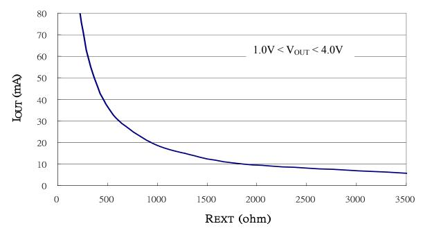
Also, when SCT2280's output voltage is set between 1.0 Volt and 4.0 Volt, the output current can be estimated approximately by :  $I_{OUT} = 30(620 / R_{EXT})$  (mA) Thus the output current are all set to be about 20.6mA at  $R_{EXT} = 900\Omega$ .
