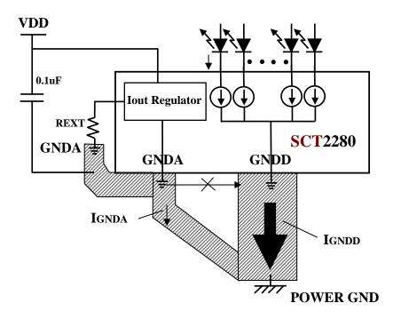
When split the ground connections, note that GNDD traces should be made shorter and wider. Maximizing the width and minimizing the length improves efficiency and ground bouncing by reducing both ground parasitic resistance and inductance. GNDA trace can be relatively narrow in application of SCT2280.
