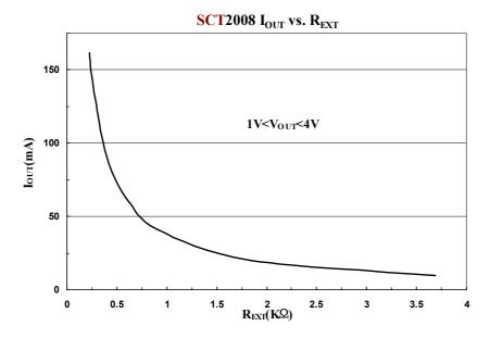
According to SCT2008' I-V curve, the output voltage should be larger than 1V to get 160 mA constant current. By applying proper output voltage, the SCT2008' output current set by an external resistor is approximate to:  $I_{OUT} = 60(630 \text{ / REXT})$  (mA) (chip skew <  $\pm 6\%$ ). Thus the output current is set to be about 42mA at REXT =  $900\Omega$ .
