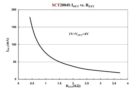
According to SCT2004S' I-V curve, the output voltage should be larger than 1V to get 180 mA constant current. By applying proper output voltage, the SCT2004S' output current set by an external resistor is approximate to:  $I_{OUT} = 120(630 / REXT)$  (mA) (chip skew <  $\pm 6\%$ ). Thus the output current is set to be about 84mA at REXT =  $900\Omega$ .
