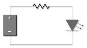
Must apply resistor(s) for protection (over current proof).
