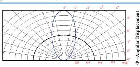
Relative Radiant Intensity vs .Angular
