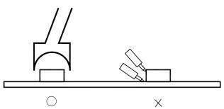
Avoid rubbing or scraping the resin by any object, during high temperature, for example reflow solder etc.
