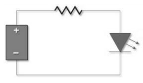
Must apply resistor(s) for protection (over current proof).
