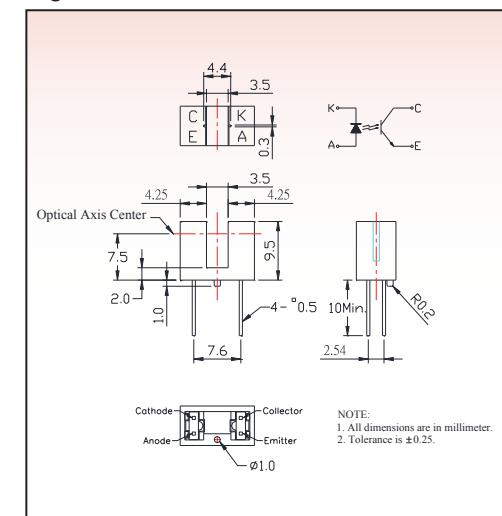
Notes: 1. All dimensions are in millimeter. 2. Tolerance is  $\pm 0.25$
