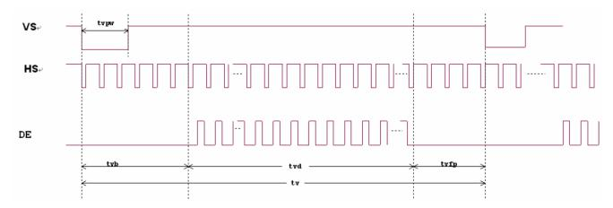
Vertical input timing diagram
