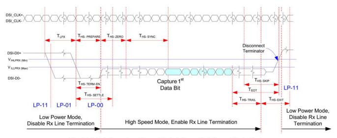
Fig. 7.3.1 Data lanes-Low Power Mode to/from High Speed Mode Timing
