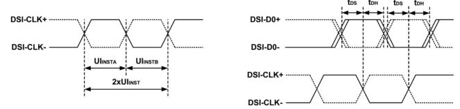
Fig. 7.1.1 DSI clock channel timing
