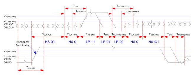
Fig. 7.3.2 Clock lanes- High Speed Mode to/from Low Power Mode Timing
