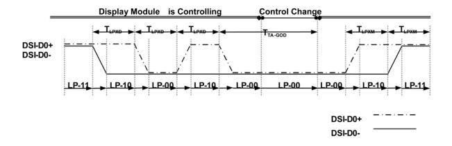
Fig. 7.2.2 Bus Turnaround (BAT) from display module to MPU Timing
