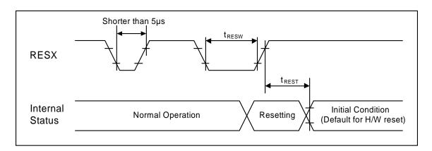
Fig. 7.4 Reset input timing
