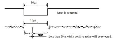
Note 5) It is necessary to wait 5msec after releasing RESX before sending commands. Also Sleep Out command cannot be sent for 120msec
