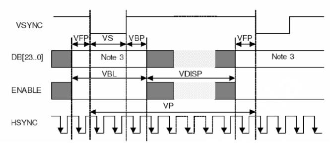
(Resolution=480x854, VSSA=VSSD=0V, VDD1=1.65V to 3.3V, VDD2=2.5 to 3.3V, VDD3=2.5 to 3.3V, T<sub>A</sub> = -30 to 70 ℃)
