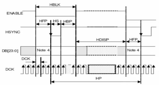
(Resolution=480x854, VSSA=VSSD=0V, VDD1=1.65V to 3.3V, VDD2=2.5 to 3.3V, VDD3=2.5 to 3.3V, T<sub>A</sub> = -30 to 70 °C)
