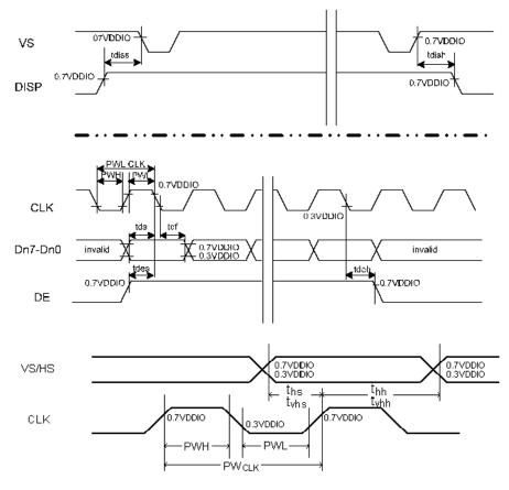
**Input Setup Timing Requirement**
