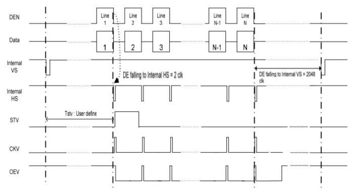
Vertical Timing Diagram DE mode(Cascade)
