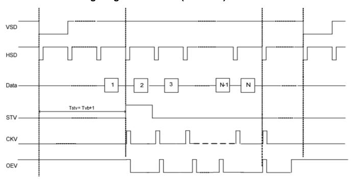
Vertical Timing Diagram HV mode(Cascade)
