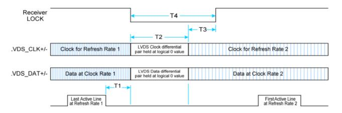
T1 - Min delay from start of vert blank to start of timing change: 2 lines (HSYNC periods)
