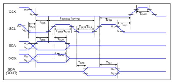
Figure 7 4-line Serial Interface Timing
